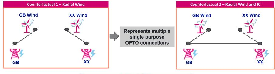
An MPI solution which integrates multiple offshore wind farms coupled with cross-border functionality
